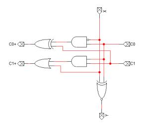
(i) Write a Verilog model to model the given 1-bit cell using primitive gates. Model the delay of AND and OR gates as 5ps, while the delay of XOR and XNOR gates as 8 ps.
