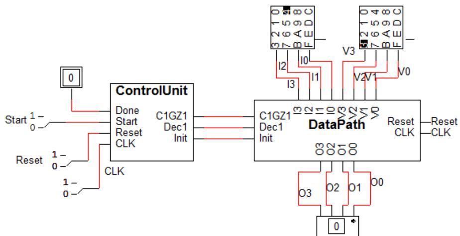
The correctness of the circuit is demonstrated in the timing diagram below where when Start is asserted the number of data values=4 is entered. The target value is set as 1. Then the values 0, 1, 2, and 3 are entered. We can see that the resulting output value is 3, which is the correct value.
