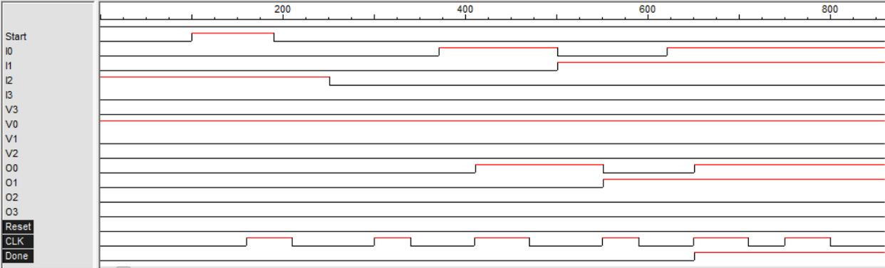
The timing diagram of another example is shown below which demonstrates that when Start is asserted, the number of data values=5 is entered. The target value is set as 4. Then the values 1, 2, 3, 4, and 5 are entered in subsequent cycles. We can see that the resulting output value is 2, which is the correct value.
