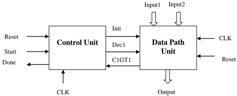
(iii) Show the design of the data-path and control unit of the circuit.
