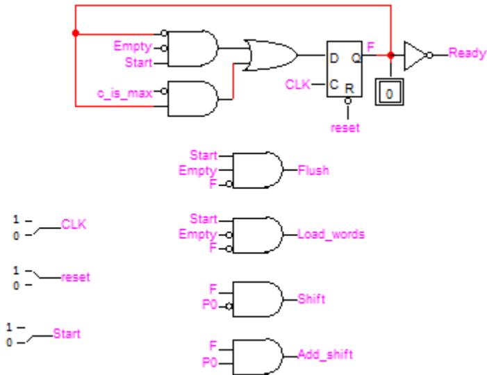
(ii) Implement the machine and verify its correct functionality by simulation.
