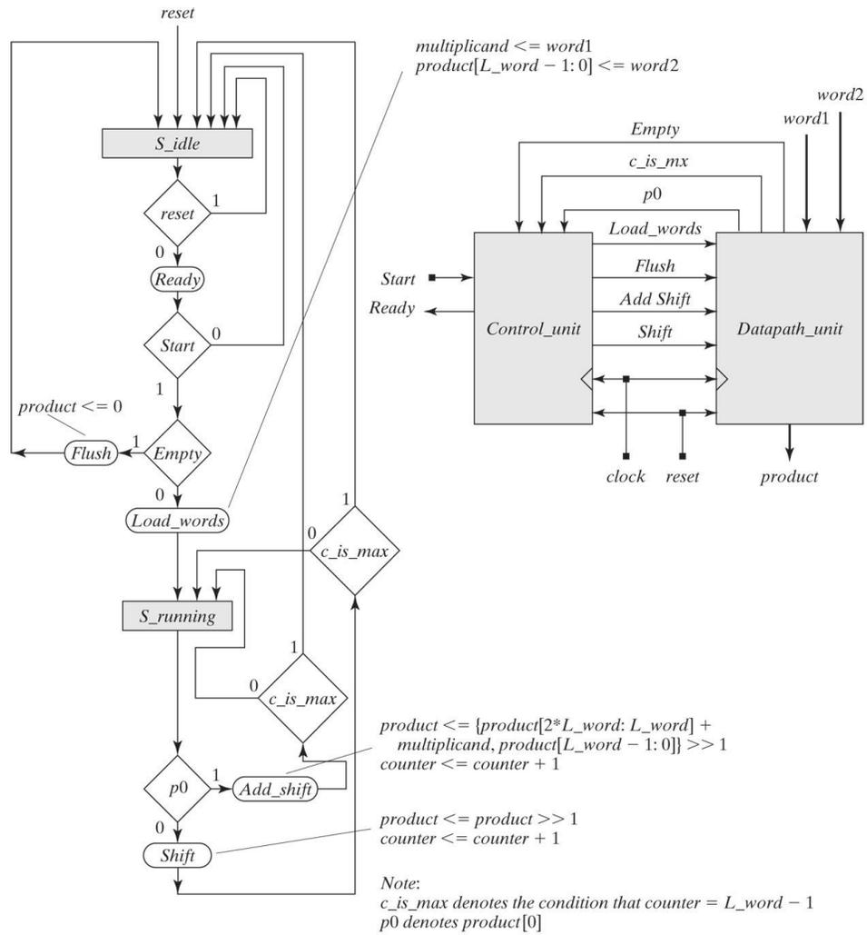
(i) Show the design of the data-path and control unit of the 4-bit sequential multiplier.
