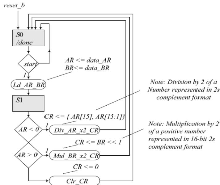
(ii) Show the design of the data-path and control unit of the machine.
