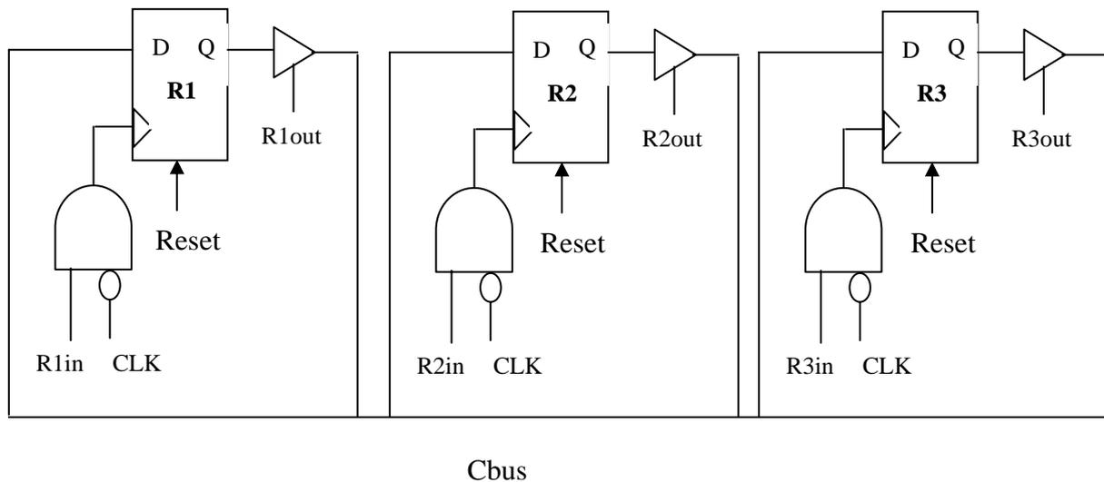
Assume that the delay across a tri-state buffer is **4 ns** and the flip-flop propagation delay is **2 ns**. Assume that the signals are of type **qit** defined as: **Type qit is ('0', '1', 'Z', 'X');**
