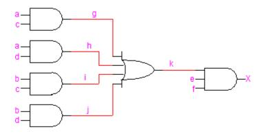
Assume that the delay of a gate is related to the number of its inputs i.e. the delay of a 2-input AND gate is 2. Also, assume that the input data-ready times are zero for all inputs except input *a*, which has a data-ready time of 2.
