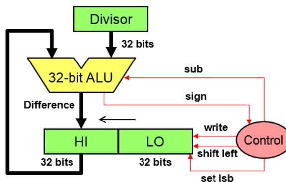
**Figure 6.5:** Sequential Binary Divider
