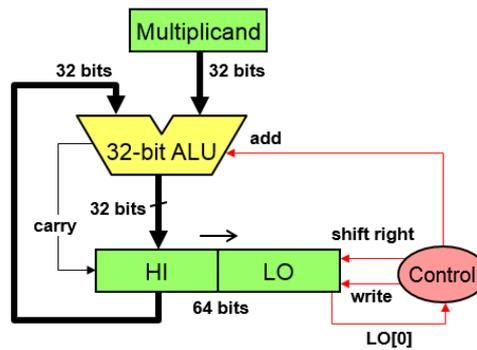
**Figure 6.2:** Sequential Binary Multiplier
