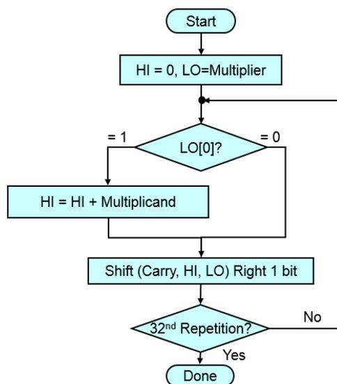
**Figure 6.1:** Sequential Binary Multiplication Algorithm
