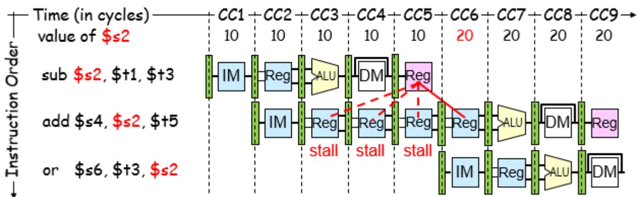
Figure 13.4: Pipeline stall due to RAW hazard.
