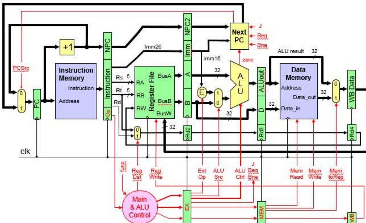
Figure 13.2: Pipeline Data Path and Control logic.
