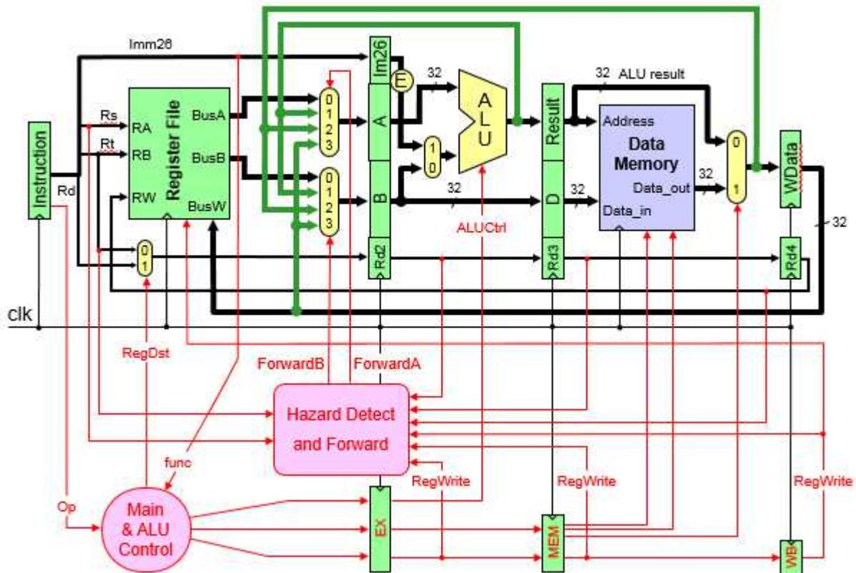
Figure 13.7: Hazard detection and forwarding unit.
