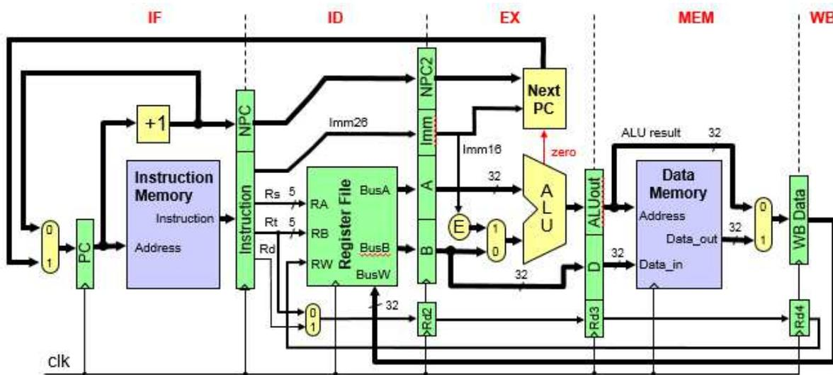
Figure 13.1: Pipelined Data Path.
