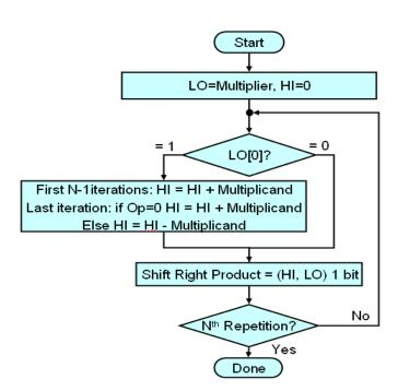
(ii) Given that Multiplicand=1010 and Multiplier=1011, using the signed multiplication hardware, show the signed multiplication of Multiplicand by Multiplier. The result of the multiplication should be an 8 bit signed number in HI and LO registers. Show the steps of your work.
