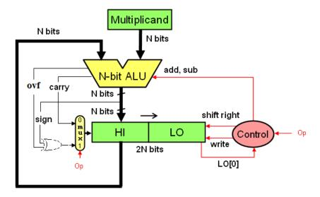
b. Show the algorithm that will be used along with your circuit in (a) for performing either signed or unsigned multiplication depending on OP.
