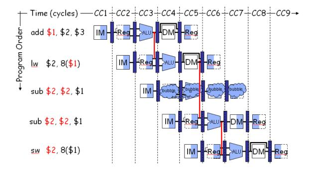
Number of clock cycles = 8. Note that in cycle 8, the execution of the sw instruction will be completed.
