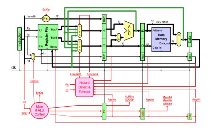
**b**) (4 **points**) Show the control signals that will be used for stalling the pipeline for data hazards due to load instructions along with their conditions. Show the necessary changes that need to be done to the design.
