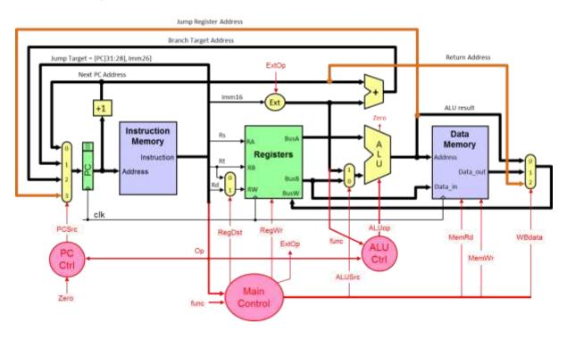
b) Same control signals are used, except that Main control logic now depends on the opcode and function code for LWI.
