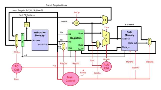
Consider adding the following two new instructions to the above datapath: JLR and LWI. The JLR instruction is I-type and has a unique opcode. The LWI instruction is R-type and has a unique function code. The least-significant 2 bits of register PC are hardwired to 00, and not stored in PC. Therefore, it is sufficient to increment PC by 1 to point to the next instruction in memory.
