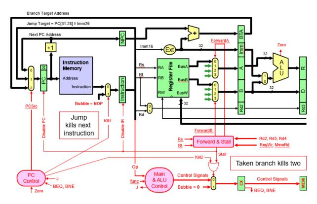
d) (3 points) Show the design of the PC control logic that includes the handling of control hazards assuming that only BEQ, BNE, and J instructions are implemented.
