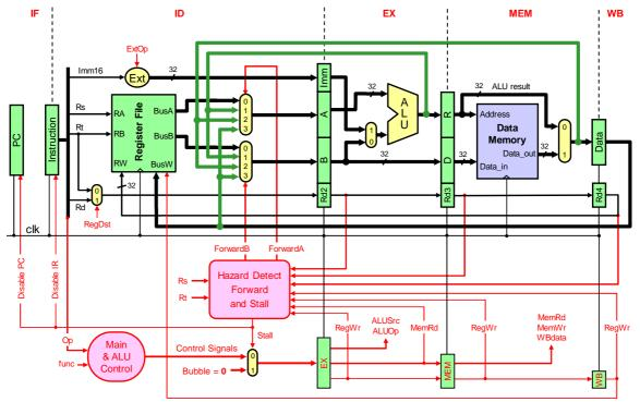
Consider the following MIPS code that is being executed on the above 5-stage pipeline:
