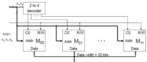
Assume three 32-bit data to be written in the above memory system at the corresponding addresses as shown in the table below:
