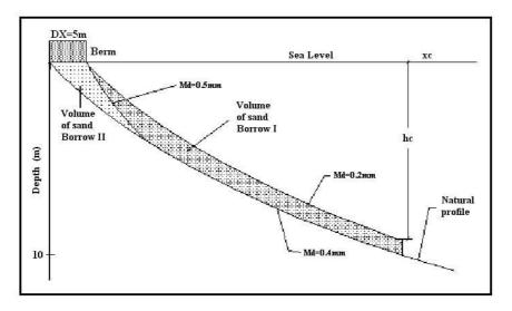
Fig. 21. Design profiles according to the mean diameter of the sand to be poured
