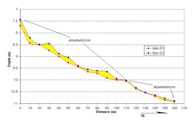
Fig. 13. Sand accumulation in the submarine slope for the action of storm waves.
