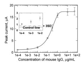
Figure 6. Dependence of anodic peak current on mouse-IgG concentration. The inset represents a magnified graph at low concentrations. The control line corresponds to the mean current in the absence of mouse IgG, and the dashed line corresponds to the mean current plus three times the standard deviation (SD).
