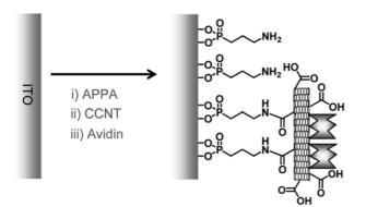
$\label{eq:Figure 1.} \textbf{Figure 1.} Schematic representation for the preparation of a CCNT/APPA/ITO electrode.$
