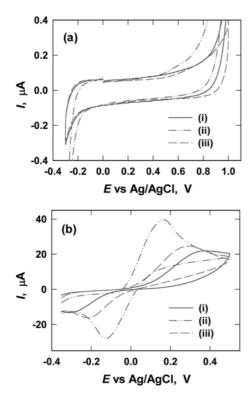
**Figure 3**. Background currents and electrocatalytic properties of modified ITO electrodes. Cyclic voltammograms of modified ITO electrodes were obtained at a scan rate of 10 mV/s in (a) a Tris buffer solution (pH 9.0) and (b) a Tris buffer solution containing 1.0 mM AP ((i) APPA/ITO electrode, (ii) CCNT/APPA/ITO electrode, and (iii) Avidin/CCNT/APPA/ITO electrode).
