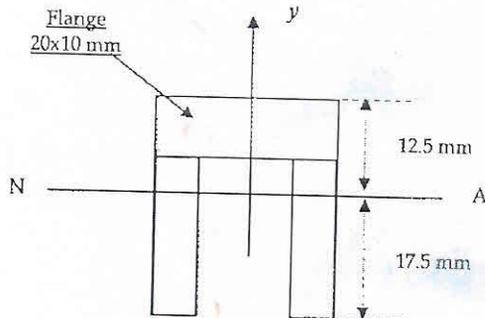
b)  $F = \sigma_{\text{avg}} \times A_{\text{flange}} = \left(\frac{\sigma_{\text{top}} + \sigma_{\text{bottom}}}{2}\right) (20 \times 10)$  (4)
