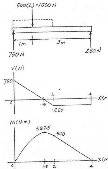
**Allowable Bending Stress:** The maximum moment is  $M_{\text{max}} = 562.5 \text{ N} \cdot \text{m}$  as indicated on the moment diagram. Applying the flexure formula
