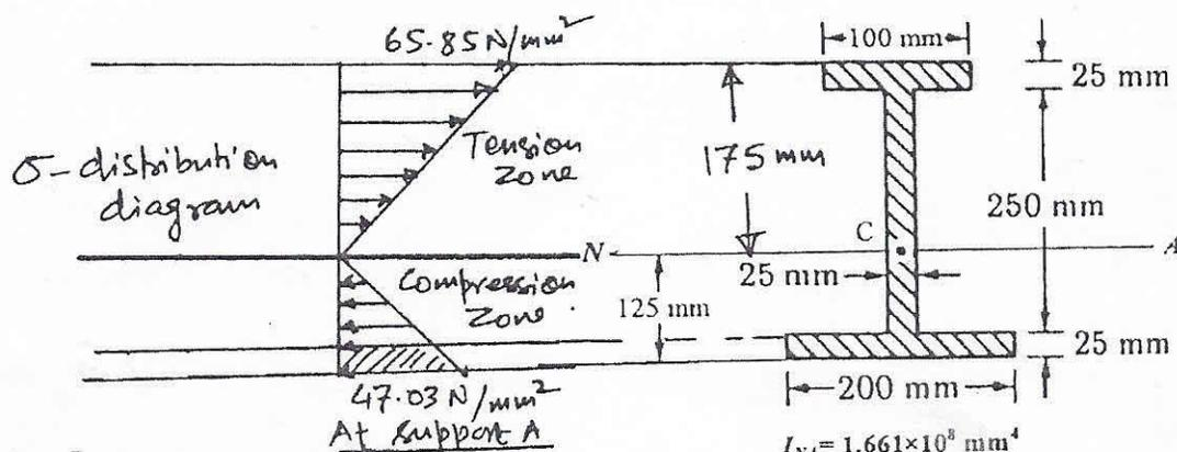
$$(a) \quad [\sigma_{\max, t}]_A = \frac{M_A C_{\text{top}}}{I_{NA}} = \frac{62.5 \times 10^6 \times 175}{1.661 \times 10^8} = 65.85 \text{ N/mm}^2 \text{ (T)}$$
