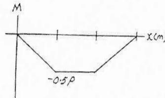
**Absolute Maximum Bending Stress:** The maximum moment is  $M_{\max} = 0.5P$  as indicated on the moment diagram. Applying the flexure formula
