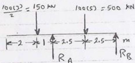
Since the distributed load has to continue to the end once it starts, we need to make equivalent load as shown below.
