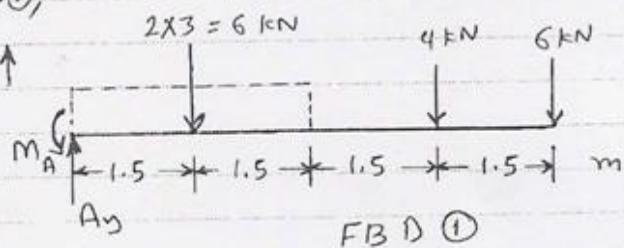
Using the singularity function, you need to remember that once the distributed load starts (from anywhere/x), it has to go all the way up to the end. (Why?) Thus, the  $2 \text{ kN/m}$ -load has to go from A to B. Therefore we have to add an upward load equals to  $2 \text{ kN/m}$  from C to B, thus making the total loads equal to the original loading. This is shown in the figure below.
