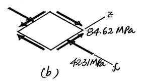
\*10–76. If the A-36 steel pipe has an outer and inner diameter of 30 mm and 20 mm, respectively, determine the factor of safety against yielding of the material at point A according to the maximum-distortion-energy theory.
