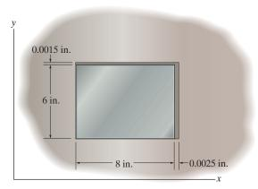
Generalized Hooke's Law: Since there are gaps between the sides of the plate and the rigid
