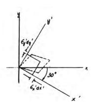
**10–11.** The state of strain at the point has components of  $\epsilon_x = -100(10^{-6})$ ,  $\epsilon_y = -200(10^{-6})$ , and  $\gamma_{xy} = 100(10^{-6})$ . Use the strain-transformation equations to determine (a) the in-plane principal strains and (b) the maximum in-plane shear strain and average normal strain. In each case specify the orientation of the element and show how the strains deform the element within the x-y plane.
