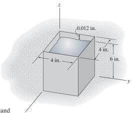
**Normal Strains:** Since the aluminum is confined at its sides by a rigid container and allowed to expand in the z direction,  $\varepsilon_x = \varepsilon_y = 0$ ; whereas  $\varepsilon_z = \frac{0.012}{6} = 0.002$ . Applying the generalized Hooke's Law with the additional thermal strain,
