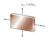
**10–82.** The state of stress acting at a critical point on the seat frame of an automobile during a crash is shown in the figure. Determine the smallest yield stress for a steel that can be selected for the member, based on the maximum-shear-stress theory.
