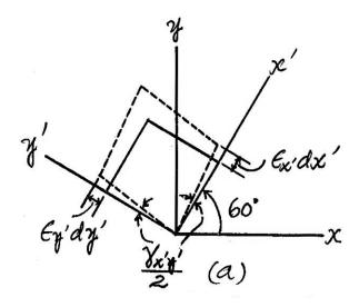
**10–7.** The state of strain at the point has components of  $\epsilon_x = 100(10^{-6})$ ,  $\epsilon_y = 300(10^{-6})$ , and  $\gamma_{xy} = -150(10^{-6})$ . Use the strain-transformation equations to determine the equivalent in-plane strains on an element oriented  $\theta = 30^{\circ}$  clockwise. Sketch the deformed element due to these strains within the x-y plane.
