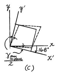
**10–27.** The 45° strain rosette is mounted on a steel shaft. The following readings are obtained from each gauge:  $\epsilon_a = 300(10^{-6})$ ,  $\epsilon_b = -250(10^{-6})$ , and  $\epsilon_c = -450(10^{-6})$ . Determine (a) the in-plane principal strains and (b) the maximum in-plane shear strain and average normal strain. In each case show the deformed element due to these strains.
