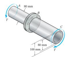
**Shear Stress.** This is a case of pure shear, and the shear stress is contributed by torsion. For the hollow segment,  $J_h = \frac{\pi}{2} \left( 0.05^4 - 0.04^4 \right) = 1.845 \pi \left( 10^{-6} \right) \text{ m}^4$ . Thus,
