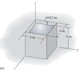
Normal Strains: Since the aluminum is confined at its sides by a rigid container, then
