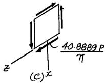
\*10–44. A single strain gauge, placed in the vertical plane on the outer surface and at an angle of 30° to the axis of the pipe, gives a reading at point A of  $\epsilon_a = -200(10^{-6})$ . Determine the principal strains in the pipe at point A. The pipe has an outer diameter of 2 in. and an inner diameter of 1 in. and is made of A-36 steel.
