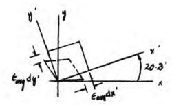
**10–6.** The state of strain at the point has components of  $\epsilon_x = -100(10^{-6})$ ,  $\epsilon_y = 400(10^{-6})$ , and  $\gamma_{xy} = -300(10^{-6})$ . Use the strain-transformation equations to determine the equivalent in-plane strains on an element oriented at an angle of  $60^{\circ}$  counterclockwise from the original position. Sketch the deformed element due to these strains within the x-y plane.
