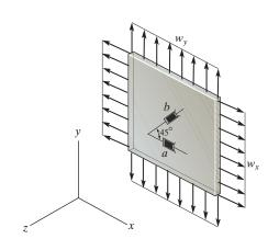
*Normal Strain:* Since no shear force acts on the plane along the x and y axes,  $\gamma_{xy}=0$ . With  $\theta_a=0$  and  $\theta_b=45^\circ$ , we have
