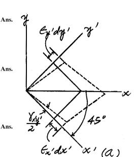
**10–13.** The state of plane strain on an element is  $\epsilon_x = -300(10^{-6})$ ,  $\epsilon_y = 0$ , and  $\gamma_{xy} = 150(10^{-6})$ . Determine the equivalent state of strain which represents (a) the principal strains, and (b) the maximum in-plane shear strain and the associated average normal strain. Specify the orientation of the corresponding elements for these states of strain with respect to the original element.
