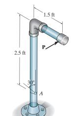
Using the method of sections and consider the equilibrium of the FBD of the pipe's upper segment, Fig. a,
