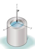
**Normal Strain:** Since the material is confined in a rigid cylinder.  $\varepsilon_x = \varepsilon_y = 0$ . Applying the generalized Hooke's Law,
