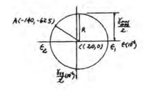
\*10–24. The strain at point A on the pressure-vessel wall has components  $\epsilon_x = 480(10^{-6})$ ,  $\epsilon_y = 720(10^{-6})$ ,  $\gamma_{xy} = 650(10^{-6})$ . Determine (a) the principal strains at A, in the x-y plane, (b) the maximum shear strain in the x-y plane, and (c) the absolute maximum shear strain.
