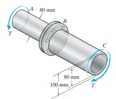
**Shear Stress:** This is a case of pure shear, and the shear stress is contributed by torsion. For the hollow segment,  $J_h = \frac{\pi}{2} \left( 0.05^4 - 0.04^4 \right) = 1.845 \pi \left( 10^{-6} \right) \text{ m}^4$ . Thus,
