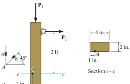
Internal Loadings: Considering the equilibrium of the free - body diagram of the post's segment, Fig. a,
