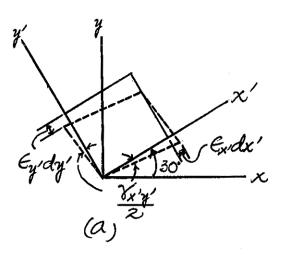
**10–3.** A strain gauge is mounted on the 1-in.-diameter A-36 steel shaft in the manner shown. When the shaft is rotating with an angular velocity of  $\omega = 1760 \text{ rev/min}$ , the reading on the strain gauge is  $\epsilon = 800(10^{-6})$ . Determine the power output of the motor. Assume the shaft is only subjected to a torque.
