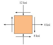
**10–79.** The yield stress for heat-treated beryllium copper is  $\sigma_Y = 130$  ksi. If this material is subjected to plane stress and elastic failure occurs when one principal stress is 145 ksi, what is the smallest magnitude of the other principal stress? Use the maximum-distortion-energy theory.
