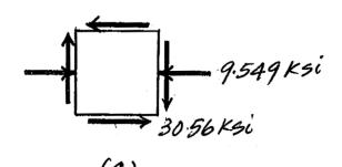
The state of stress at the points on the surface of the shaft is represented on the element shown in Fig. a.
