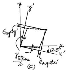
\*10–28. The 45° strain rosette is mounted on the link of the backhoe. The following readings are obtained from each gauge:  $\epsilon_a = 650(10^{-6})$ ,  $\epsilon_b = -300(10^{-6})$ ,  $\epsilon_c = 480(10^{-6})$ . Determine (a) the in-plane principal strains and (b) the maximum in-plane shear strain and associated average normal strain.
