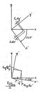
\*10–16. The state of strain at a point on a support has components of  $\epsilon_x = 350(10^{-6})$ ,  $\epsilon_y = 400(10^{-6})$ ,  $\gamma_{xy} = -675(10^{-6})$ . Use the strain-transformation equations to determine (a) the in-plane principal strains and (b) the maximum in-plane shear strain and average normal strain. In each case specify the orientation of the element and show how the strains deform the element within the x-y plane.
