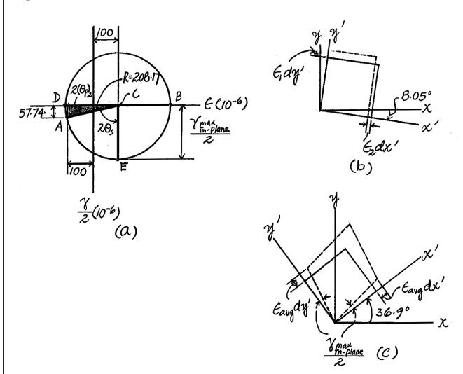
**10–26.** The  $60^{\circ}$  strain rosette is mounted on a beam. The following readings are obtained for each gauge:  $\epsilon_a = 200(10^{-6})$ ,  $\epsilon_b = -450(10^{-6})$ , and  $\epsilon_c = 250(10^{-6})$ . Determine (a) the in-plane principal strains and (b) the maximum in-plane shear strain and average normal strain. In each case show the deformed element due to these strains.
