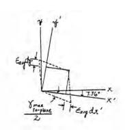
10-22. The strain at point A on the bracket has components  $\epsilon_x = 300(10^{-6}), \quad \epsilon_y = 550(10^{-6}), \quad \gamma_{xy} =$  $-650(10^{-6})$ . Determine (a) the principal strains at A in the x-y plane, (b) the maximum shear strain in the x-y plane, and (c) the absolute maximum shear strain.
