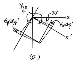
\*10–8. The state of strain at the point on the bracket has components  $\epsilon_x = -200(10^{-6})$ ,  $\epsilon_y = -650(10^{-6})$ ,  $\gamma_{xy} = -175(10^{-6})$ . Use the strain-transformation equations to determine the equivalent in-plane strains on an element oriented at an angle of  $\theta = 20^{\circ}$  counterclockwise from the original position. Sketch the deformed element due to these strains within the x-y plane.
