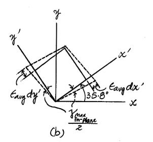
**10–10.** The state of strain at the point on the bracket has components  $\epsilon_x = 400(10^{-6})$ ,  $\epsilon_y = -250(10^{-6})$ ,  $\gamma_{xy} = 310(10^{-6})$ . Use the strain-transformation equations to determine the equivalent in-plane strains on an element oriented at an angle of  $\theta = 30^{\circ}$  clockwise from the original position. Sketch the deformed element due to these strains within the x-y plane.
