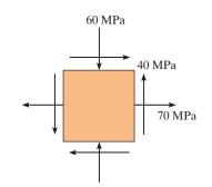
\*10-72. The components of plane stress at a critical point on an A-36 steel shell are shown. Determine if failure (yielding) has occurred on the basis of the maximum-distortion-energy theory.
