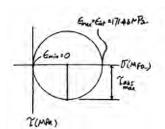
\*10–40. The strain in the x direction at point A on the steel beam is measured and found to be  $\epsilon_x = -100(10^{-6})$ . Determine the applied load P. What is the shear strain  $\gamma_{xy}$  at point A?  $E_{\rm st} = 29(10^3)$  ksi,  $\nu_{\rm st} = 0.3$ .
