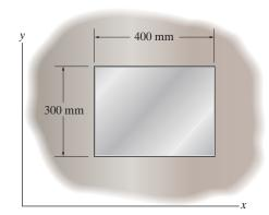
Generalized Hooke's Law: Since the sides of the aluminum plate are confined in the rigid constraint along the x and y directions,  $\varepsilon_x = \varepsilon_y = 0$ . However, the plate is allowed to have free expansion along the z direction. Thus,  $\sigma_z = 0$ . With the additional thermal strain term, we have
