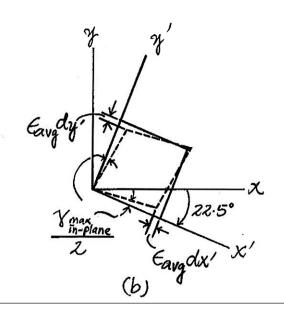
\*10-12. The state of plane strain on an element is given by  $\epsilon_x = 500(10^{-6}), \ \epsilon_y = 300(10^{-6}), \ \text{and} \ \gamma_{xy} = -200(10^{-6}).$ Determine the equivalent state of strain on an element at the same point oriented 45° clockwise with respect to the original element.
