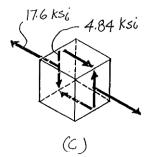
**8–58.** The 2-in.-diameter rod is subjected to the loads shown. Determine the state of stress at point B, and show the results on a differential element located at this point.
