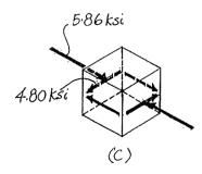
**8–59.** If P = 60 kN, determine the maximum normal stress developed on the cross section of the column.
