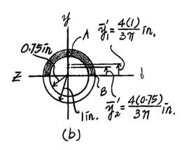
**8–66.** Determine the state of stress at point B on the cross section of the pipe at section a-a.
