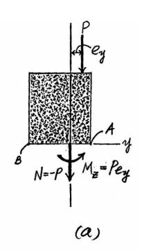
\*8–68. The bar has a diameter of 40 mm. If it is subjected to a force of  $800 \,\mathrm{N}$  as shown, determine the stress components that act at point A and show the results on a volume element located at this point.
