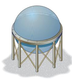
**Normal Stress:** Since  $\frac{r}{t} = \frac{4}{0.03} = 133.33 > 10$ , thin-wall analysis is valid. For the spherical tank's wall,
