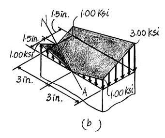
**8–46.** The support is subjected to the compressive load **P**. Determine the absolute maximum and minimum normal stress acting in the material.
