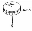
**8–86.** The cap on the cylindrical tank is bolted to the tank along the flanges. The tank has an inner diameter of 1.5 m and a wall thickness of 18 mm. If the pressure in the tank is p=1.20 MPa, determine the force in each of the 16 bolts that are used to attach the cap to the tank. Also, specify the state of stress in the wall of the tank.
