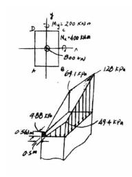
**8–55.** The bar has a diameter of 40 mm. If it is subjected to the two force components at its end as shown, determine the state of stress at point A and show the results on a differential volume element located at this point.
