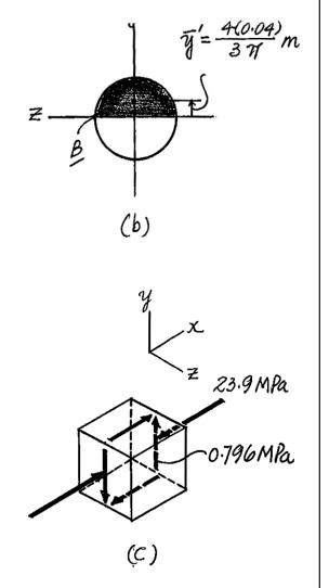
\*8–44. Determine the normal stress developed at points A and B. Neglect the weight of the block.
