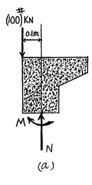
\*8–20. Determine the maximum and minimum normal stress in the bracket at section a–a when the load is applied at x = 300 mm.
