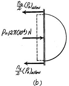
Referring to the free-body diagram of the hemispherical cap, Fig. b, where  $P = pA = 3(10^6) \left[ \frac{\pi}{4} (4^2) \right] = 12\pi (10^6) \text{ N},$
