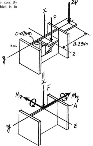
•8–61. The beveled gear is subjected to the loads shown. Determine the stress components acting on the shaft at point A, and show the results on a volume element located at this point. The shaft has a diameter of 1 in. and is fixed to the wall at C.
