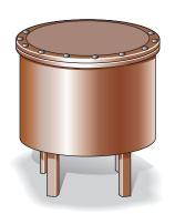
**Hoop Stress for Cylindrical Tank:** Since  $\frac{r}{t} = \frac{750}{18} = 41.7 > 10$ , then thin wall analysis can be used. Applying Eq. 8–1
