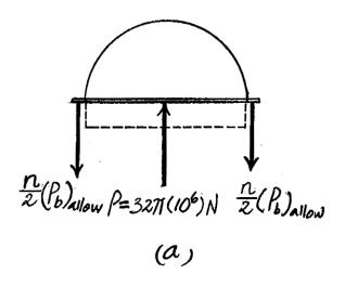
**8–7.** A boiler is constructed of 8-mm thick steel plates that are fastened together at their ends using a butt joint consisting of two 8-mm cover plates and rivets having a diameter of 10 mm and spaced 50 mm apart as shown. If the steam pressure in the boiler is 1.35 MPa, determine (a) the circumferential stress in the boiler's plate apart from the seam, (b) the circumferential stress in the outer cover plate along the rivet line *a*–*a*, and (c) the shear stress in the rivets.
