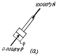
•8–81. The hydraulic cylinder has an inner diameter of 100 mm and wall thickness of t=4 mm. If it is made from a material having an allowable normal stress of  $\sigma_{\rm allow}=150$  MPa, determine the maximum allowable force **P**.
