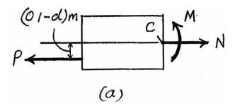
\*8–32. The horizontal force of  $P=80~\mathrm{kN}$  acts at the end of the plate. The plate has a thickness of 10 mm and  $\mathbf{P}$  acts along the centerline of this thickness such that  $d=50~\mathrm{mm}$ . Plot the distribution of normal stress acting along section a–a.
