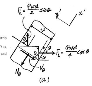
**8–17.** In order to increase the strength of the pressure vessel, filament winding of the same material is wrapped around the circumference of the vessel as shown. If the pretension in the filament is T and the vessel is subjected to an internal pressure p, determine the hoop stresses in the filament and in the wall of the vessel. Use the free-body diagram shown, and assume the filament winding has a thickness t' and width w for a corresponding length of the vessel.
