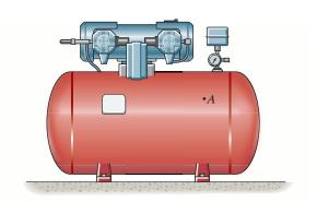
*Hoop Stress for Cylindrical Vessels:* Since  $\frac{r}{t} = \frac{11}{0.25} = 44 > 10$ , then *thin wall* analysis can be used. Applying Eq. 8–1
