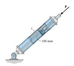
**Equation of Equilibrium:** The absolute pressure developed in the hydraulic cylinder can be determined by considering the equilibrium of the free-body diagram of the piston shown in Fig. a. The resultant force of the pressure on the piston is  $F = pA = p \left[ \frac{\pi}{4} \left( 0.1^2 \right) \right] = 0.0025 \pi p$ . Thus,
