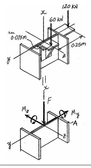
\*8–60. Determine the maximum allowable force **P**, if the column is made from material having an allowable normal stress of  $\sigma_{\rm allow} = 100$  MPa.
