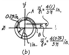
•8–67. The eccentric force **P** is applied at a distance  $e_y$  from the centroid on the concrete support shown. Determine the range along the y axis where **P** can be applied on the cross section so that no tensile stress is developed in the material.
