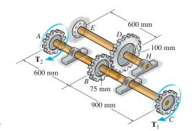
Equilibrium: Referring to the free - body diagram of shaft ABC shown in Fig. a
