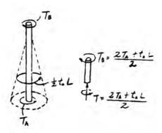
**5–30.** The shaft is subjected to a distributed torque along its length of  $t = (10x^2) \,\mathrm{N} \cdot \mathrm{m/m}$ , where x is in meters. If the maximum stress in the shaft is to remain constant at 80 MPa, determine the required variation of the radius c of the shaft for  $0 \le x \le 3$  m.
