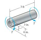
**Elastic - Plastic Torque.** The shear stress distribution due to **T** is shown in Fig. *a*. The linear portion of this distribution can be expressed as  $\tau = \frac{10}{2.25}\rho = 4.444\rho$ . Thus,  $\tau_{\rho=1.5\,\mathrm{in.}} = 4.444(1.5) = 6.667\,\mathrm{ksi.}$
