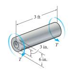
**Plastic Torque**. When the inner surface of the shaft is about to yield, the shaft is about to become fully plastic.
