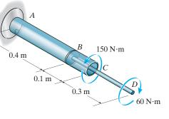
$$\phi_D = \sum \frac{T_i L_i}{J_i G_i} = \frac{T_{AB} L_{AB}}{J_{AB} G_{st}} + \frac{T_{BD} L_{BD}}{J_{BD} G_{st}}$$
