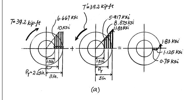
**5–139.** The tube is made of elastic-perfectly plastic material, which has the  $\tau-\gamma$  diagram shown. Determine the torque T that just causes the inner surface of the shaft to yield. Also, find the residual shear-stress distribution in the shaft when the torque is removed.
