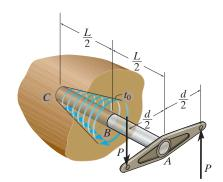
**Internal Loading:** The distributed torque expressed as a function of x, measured from the left end, is  $t = \left(\frac{t_o}{L/2}\right)x = \left(\frac{4Pd/L}{L/2}\right)x = \left(\frac{8Pd}{L^2}\right)x$ . Thus, the resultant torque within region x of the shaft i
