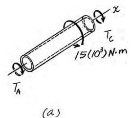
\*5–136. The tubular shaft is made of a strain-hardening material having a  $\tau$ - $\gamma$  diagram as shown. Determine the torque T that must be applied to the shaft so that the maximum shear strain is 0.01 rad.
