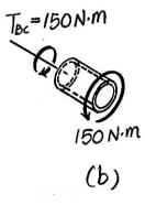
**5–55.** The assembly is made of A-36 steel and consists of a solid rod 20 mm in diameter fixed to the inside of a tube using a rigid disk at *B*. Determine the angle of twist at *C*. The tube has an outer diameter of 40 mm and wall thickness of 5 mm.
