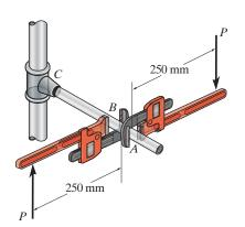
Internal Loading: By observation, segment BC of the pipe is critical since it is subjected to a greater internal torque than segment AB. Writing the moment equation of equilibrium about the x axis by referring to the free-body diagram shown in Fig. a, we have
