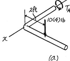
**5–18.** The rod has a diameter of 1 in. and a weight of 15 lb/ft. Determine the maximum torsional stress in the rod at a section located at B due to the rod's weight.
