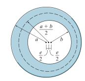
•5–113. The mean dimensions of the cross section of an airplane fuselage are shown. If the fuselage is made of 2014-T6 aluminum alloy having allowable shear stress of  $\tau_{\rm allow} = 18$  ksi, and it is subjected to a torque of 6000 kip • ft, determine the required minimum thickness t of the cross section to the nearest 1/16 in. Also, find the corresponding angle of twist per foot length of the fuselage.
