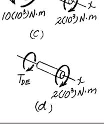
\*5-72. The 80-mm diameter shaft is made of 6061-T6 aluminum alloy and subjected to the torsional loading shown. Determine the angle of twist at end A.
