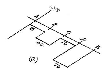
\*5–16. The solid shaft has a diameter of 40 mm. Determine the absolute maximum shear stress in the shaft and sketch the shear-stress distribution along a radial line of the shaft where the shear stress is maximum.
