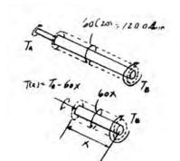
\*5–92. If the shaft is subjected to a uniform distributed torque of  $t = 20 \text{ kN} \cdot \text{m/m}$ , determine the maximum shear stress developed in the shaft. The shaft is made of 2014-T6 aluminum alloy and is fixed at A and C.
