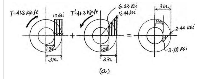
\*5–140. The 2-m-long tube is made of an elastic-perfectly plastic material as shown. Determine the applied torque T that subjects the material at the tube's outer edge to a shear strain of  $\gamma_{\rm max} = 0.006$  rad. What would be the permanent angle of twist of the tube when this torque is removed? Sketch the residual stress distribution in the tube.
