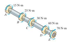
The internal torques developed in each segment of the shaft are shown in the torque diagram, Fig. a.
