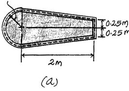
**5–119.** The symmetric tube is made from a high-strength steel, having the mean dimensions shown and a thickness of 5 mm. If it is subjected to a torque of  $T=40~\mathrm{N}\cdot\mathrm{m}$ , determine the average shear stress developed at points A and B. Indicate the shear stress on volume elements located at these points.
