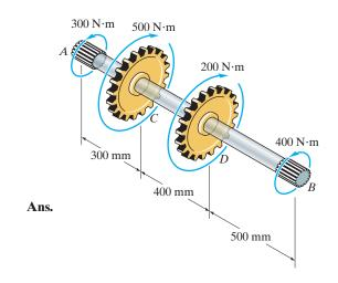
•5–57. The motor delivers 40 hp to the 304 stainless steel shaft while it rotates at 20 Hz. The shaft is supported on smooth bearings at A and B, which allow free rotation of the shaft. The gears C and D fixed to the shaft remove 25 hp and 15 hp, respectively. Determine the diameter of the shaft to the nearest  $\frac{1}{8}$  in. if the allowable shear stress is  $\tau_{\rm allow}=8$  ksi and the allowable angle of twist of C with respect to D is  $0.20^{\circ}$ .
