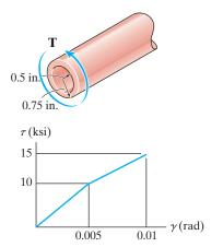
From the shear-strain diagram,
