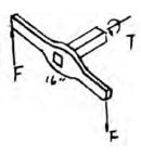
**5–106.** The steel shaft is 12 in. long and is screwed into the wall using a wrench. Determine the maximum shear stress in the shaft and the amount of displacement that each couple force undergoes if the couple forces have a magnitude of F=30 lb,  $G_{\rm st}=10.8(10^3)$  ksi.
