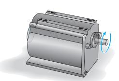
**5–34.** The gear motor can develop 3 hp when it turns at 150 rev/min. If the allowable shear stress for the shaft is  $\tau_{\rm allow} = 12$  ksi, determine the smallest diameter of the shaft to the nearest  $\frac{1}{8}$  in. that can be used.
