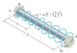
$$T(x) = \int_0^x t_0 \left( 1 + \frac{x^2}{L^2} \right) dx = t_0 \left( x + \frac{x^2}{3L^2} \right)$$
