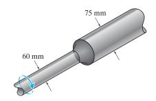
**5–123.** The steel shaft is made from two segments: AB and BC, which are connected using a fillet weld having a radius of 2.8 mm. Determine the maximum shear stress developed in the shaft.
