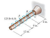
Maximum Shear Stress: Applying the torsion formula
