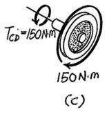
**5–15.** The solid shaft is made of material that has an allowable shear stress of  $\tau_{\rm allow}=10$  MPa. Determine the required diameter of the shaft to the nearest mm.
