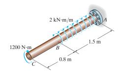
The internal torque for segment BC is Constant  $T_{BC} = 1200 \text{ N} \cdot \text{m}$ , Fig. a. However, the internal for segment AB varies with x, Fig. b.
