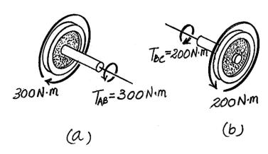
\*5–28. The A-36 steel shaft is supported on smooth bearings that allow it to rotate freely. If the gears are subjected to the torques shown, determine the required diameter of the shaft to the nearest mm if  $\tau_{\rm allover} = 60$  MPa.
