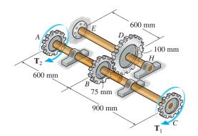
Equilibrium: Referring to the free - body diagram of shaft ABC shown in Fig. a
