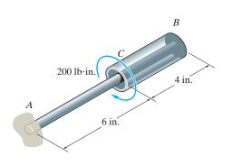
$$\phi_B = \frac{T_{AB}L}{JG} = \frac{200(10)}{\frac{\pi}{2}(0.5)^4(11.0)(10^6)} = 0.001852 \text{ rad}$$
