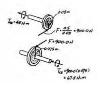
•5–69. The shafts are made of A-36 steel and each has a diameter of 80 mm. Determine the angle of twist at end E.
