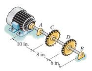
**External Applied Torque:** Applying  $T = \frac{P}{2\pi f}$ , we have
