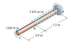
The internal torque for segment BC is constant  $T_{BC} = 1200 \text{ N} \cdot \text{m}$ , Fig. a. However, the internal torque for segment AB varies with x, Fig. b.
