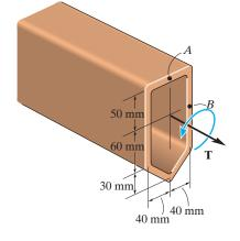
•5–117. The mean dimensions of the cross section of the leading edge and torsion box of an airplane wing can be approximated as shown. If the wing is made of 2014-T6 aluminum alloy having an allowable shear stress of  $\tau_{\rm allow}=125$  MPa and the wall thickness is 10 mm, determine the maximum allowable torque and the corresponding angle of twist per meter length of the wing.
