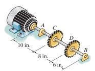
**External Applied Torque:** Applying  $T = \frac{P}{2\pi f}$ , we have
