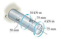
The internal torques developed at Cross-sections pass through point B and A are shown in Fig. a and b, respectively.
