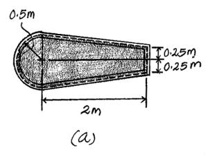
**5–118.** The mean dimensions of the cross section of the leading edge and torsion box of an airplane wing can be approximated as shown. If the wing is subjected to a torque of  $4.5~\mathrm{MN}\cdot\mathrm{m}$  and the wall thickness is 10 mm, determine the average shear stress developed in the wing and the angle of twist per meter length of the wing. The wing is made of 2014-T6 aluminum alloy.
