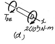
5-70. The shafts are made of A-36 steel and each has a diameter of 80 mm. Determine the angle of twist of gear D.
