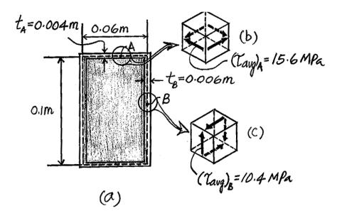
\*5–116. The tube is made of plastic, is 5 mm thick, and has the mean dimensions shown. Determine the average shear stress at points A and B if it is subjected to the torque of  $T = 5 \,\mathrm{N} \cdot \mathrm{m}$ . Show the shear stress on volume elements located at these points.
