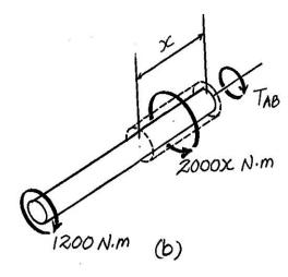
**5–22.** The solid shaft is subjected to the distributed and concentrated torsional loadings shown. Determine the required diameter d of the shaft to the nearest mm if the allowable shear stress for the material is  $\tau_{\rm allow} = 50 \, {\rm MPa}$ .
