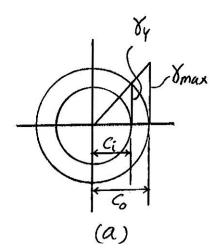
5-135. The hollow shaft has inner and outer diameters of 60 mm and 80 mm, respectively. If it is made of an elasticperfectly plastic material, which has the  $\tau - \gamma$  diagram shown, determine the reactions at the fixed supports A and C.
