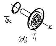
\*5–68. The 30-mm-diameter shafts are made of L2 tool steel and are supported on journal bearings that allow the shaft to rotate freely. If the motor at A develops a torque of  $T=45~\mathrm{N}\cdot\mathrm{m}$  on the shaft AB, while the turbine at E is fixed from turning, determine the amount of rotation of gears B and C.
