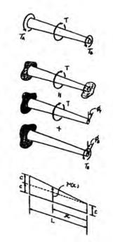
**5–94.** The shaft of radius c is subjected to a distributed torque t, measured as torque/length of shaft. Determine the reactions at the fixed supports A and B.
