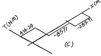
**5–79.** The steel shaft is made from two segments: AC has a diameter of 0.5 in, and CB has a diameter of 1 in. If it is fixed at its ends A and B and subjected to a torque of determine the maximum shear stress in the shaft.  $G_{\rm st}=10.8(10^3)$  ksi.
