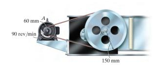
*Internal Torque:* For shafts A and B
