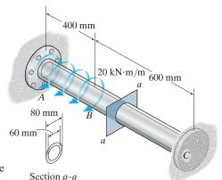
**Equilibrium:** Referring to the free - body diagram of the shaft shown in Fig. a, we have
