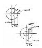
•5–137. The shear stress–strain diagram for a solid 50-mm-diameter shaft can be approximated as shown in the figure. Determine the torque *T* required to cause a maximum shear stress in the shaft of 125 MPa. If the shaft is 1.5 m long, what is the corresponding angle of twist?
