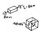
\*5–104. The 6061-T6 aluminum bar has a square cross section of 25 mm by 25 mm. If it is 2 m long, determine the maximum shear stress in the bar and the rotation of one end relative to the other end.
