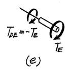
•5–89. The shafts are made of A-36 steel and have the same diameter of 4 in. If a torque of 15 kip  $\cdot$  ft is applied to gear B, determine the angle of twist of gear B.
