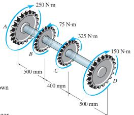
The internal torque developed in segments AB , BC and CD of the shaft are shown in Figs. a, b and c.
