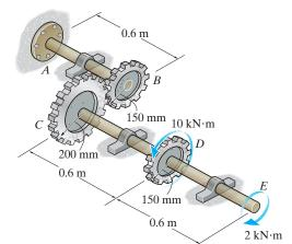
Equilibrium: Referring to the free - body diagram of shaft CDE shown in Fig. a,
