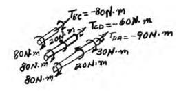
**5–54.** The assembly is made of A-36 steel and consists of a solid rod 20 mm in diameter fixed to the inside of a tube using a rigid disk at B. Determine the angle of twist at D. The tube has an outer diameter of 40 mm and wall thickness of 5 mm.
