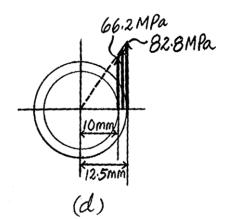
\*5-20. Two wrenches are used to tighten the pipe. If the pipe is made from a material having an allowable shear stress of  $\tau_{\rm allow} = 85$  MPa, determine the allowable maximum force P that can be applied to each wrench. The pipe has an outer diameter of 25 mm and inner diameter of 20 mm.
