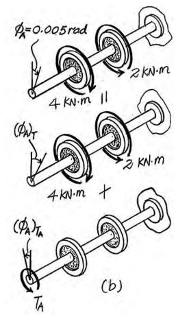
•5–81. The shaft is made of A-36 steel and has a diameter of 80 mm. It is fixed at B and the support at A has a torsional stiffness of  $k=0.5 \, \mathrm{MN} \cdot \mathrm{m/rad}$ . If it is subjected to the gear torques shown, determine the absolute maximum shear stress in the shaft.
