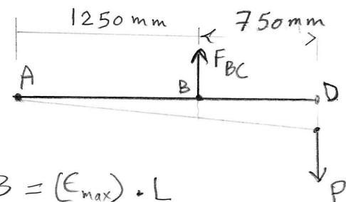
$$\Rightarrow \text{The max. allow displacement of B} = (\epsilon_{max})_{BC} \cdot L_{BC} \\ = (0.8 \times 10^{-3} \frac{\text{mm}}{\text{mm}}) \cdot (1000 \text{ mm}) \\ = 0.8 \text{ mm} < 2.5 \text{ mm}$$
