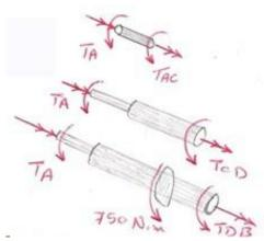
Note that all internal torques are assumed (+). Also note that the right part of segment DB may be chosen as shown.
