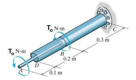
3 - The given hollow circular shaft is subjected to the distributed and concentrated torsional loadings shown. Determine the absolute maximum shear stresses in BC, and the absolute maximum shear stresses in BA. Sketch a diagram for the value of the internal torque  $T_R$  along axis CA. (outer radius = 50 mm, inner radius = 30 mm)
