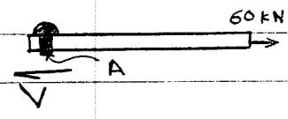
Note: there is only one rivet, and it is in single shear.
