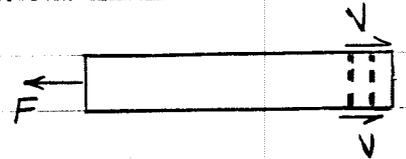
$$\tau_{ave} = \frac{V}{A} \Rightarrow 110 \equiv \frac{F}{2(6)(\frac{\pi}{4})(4)^2} \quad \text{double shear} \quad \text{six pins} \quad \text{area of each pin}$$
