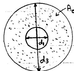
Note that the bearing stress is reduced a lot by adding a washer (28.29 vs. 106.1 MPa).
