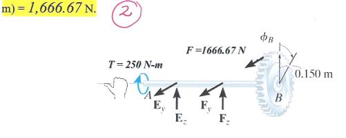
Summing moment about the x-axis of shaft DC, the force F = 1,666.67 N creates the torque react at the fixed end D;  $T_D = (1,666.67 \text{ N})(0.075 \text{ m})$ .
