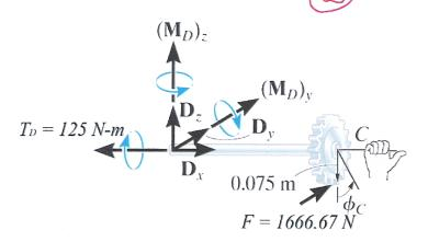
Maximum shear stress due to an applied torque;  $\tau_{max} = TC/J$
