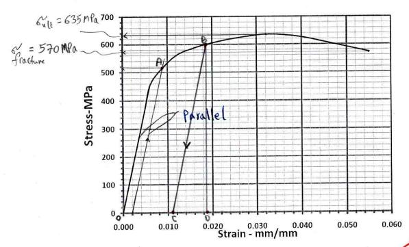
The modulus of elasticity, E = 300 MPa - 0 = 75 X 10 Pa. 3
