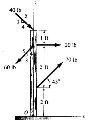
$$\begin{aligned}\sum F_y &= 70 \sin 45^\circ - 40\left(\frac{3}{5}\right) - 60\left(\frac{4}{5}\right) \\ &= -22.50 \text{ lb} = 22.50 \text{ lb} \downarrow\end{aligned}$$
