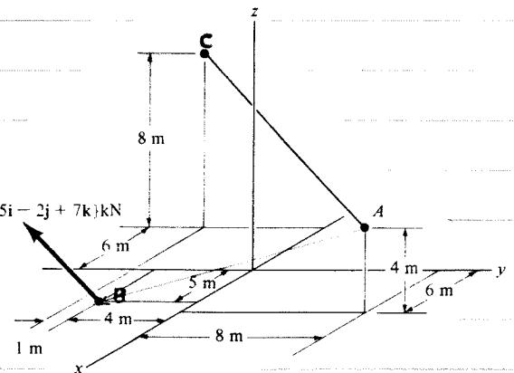
$$\Rightarrow M_{AC} = \begin{vmatrix} u_{AC}^x & u_{AC}^y & u_{AC}^z \\ r_x & r_y & r_z \\ F_x & F_y & F_z \end{vmatrix} = \begin{vmatrix} -0.6616 & -0.7167 & 0.2205 \\ -1 & -12 & -4 \\ 0.5 & -2 & 7 \end{vmatrix}$$
