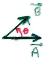
Thus, the dot product is the product of the magnitudes of  $\vec{A}$  and  $\vec{B}$  and of the cosine of the angle  $\theta$  formed by  $\vec{A}$  and  $\vec{B}$ .
