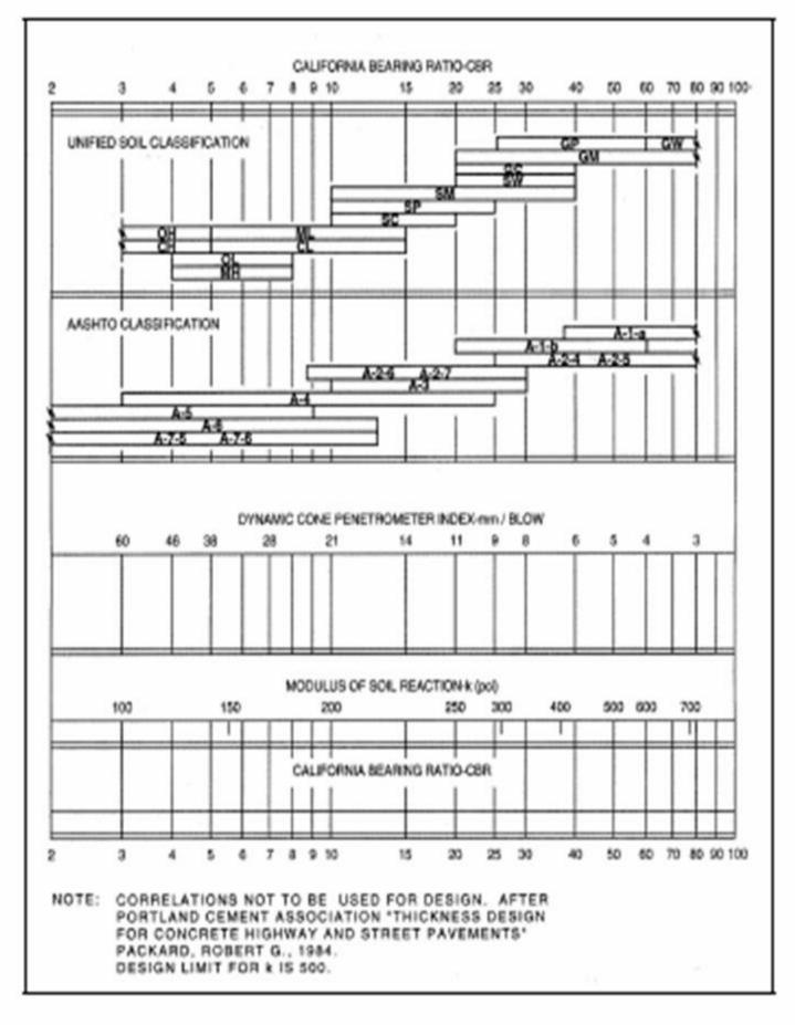
Figure 5-3. Approximate relationships of soil classification and soil strength
