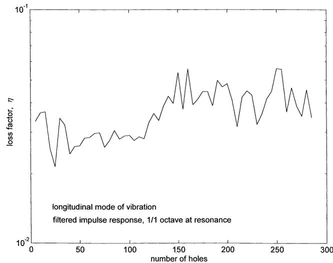
Fig. 8. Variation of the loss factor with the number of defects in the wooden bar.
