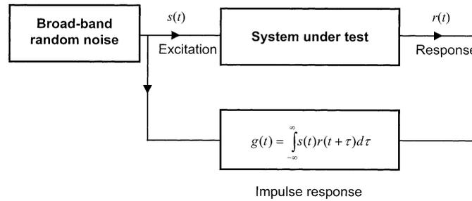
Fig. 3. Measurement of the impulse response of a system by a method based on a cross-correlation principle.
