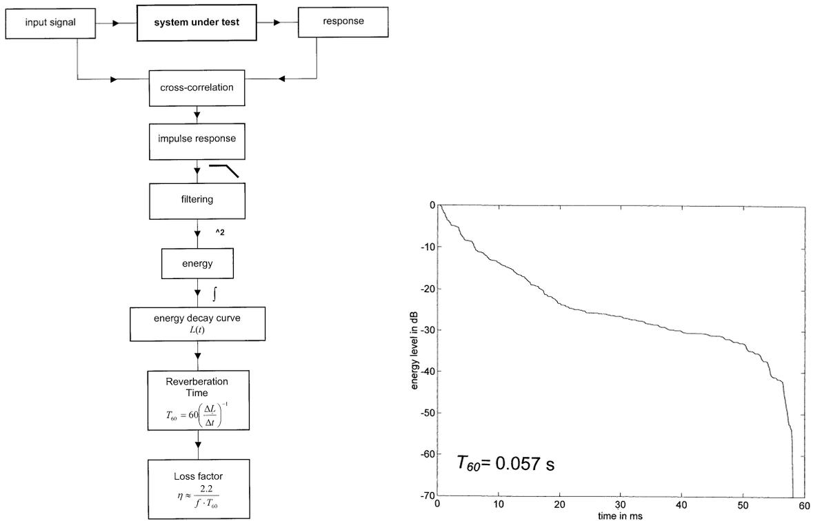
Fig. 4. Left: representation of a procedure for the measurement of the loss factor of a material specimen. Right: a typical energy decay curve resulting from the application of the integrated impulse response method.
