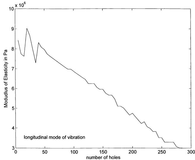
Fig. 7. Variation of the MOE as function of the number of holes drilled in the wooden bar.
