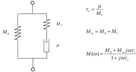
Fig. 2. The Zener model, also known as the standard viscoelastic body.
