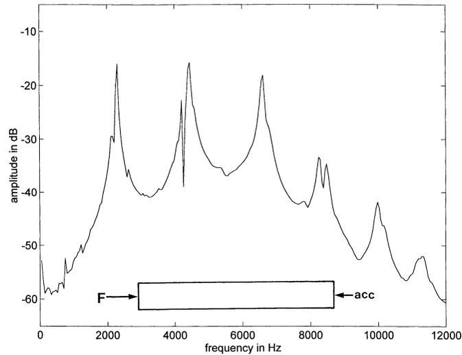
Fig. 6. Frequency response of the wooden bar submitted to a longitudinal vibration excitation.
