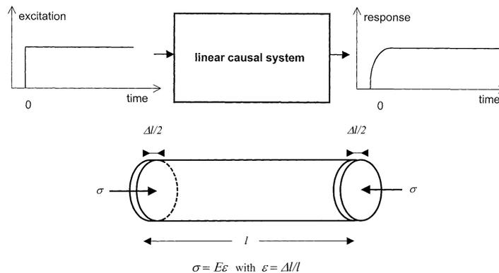
Fig. 1. Representation of the MOE of a material as the frequency response of a sample of this material.
