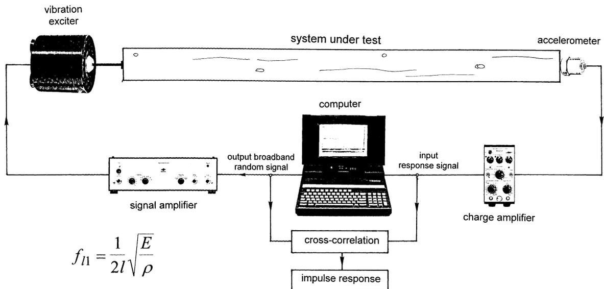
Fig. 5. Schematic representation of the experimental set-up for assessing the vibration impulse response of a test specimen in the longitudinal mode of vibration.
