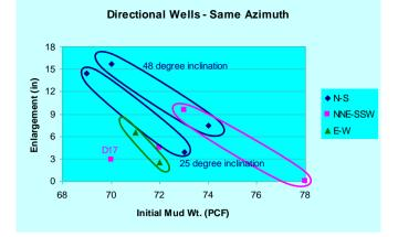
Figure 9. Hole enlargement versus initial mud weight of directional wells studied with respect to azimuth.
