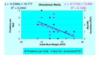
Figure 7. Problems per well and mud weight increment versus initial mud weight of directional wells.
