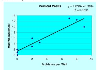
Figure 3. Mud weight increment versus problems per well of vertical wells.
