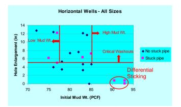
Figure 11. Hole enlargement versus initial mud weight of horizontal wells showing stuck pipes – definition of critical washouts.
