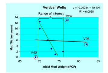
Figure 2. Mud weight increment versus initial mud weight of vertical wells.
