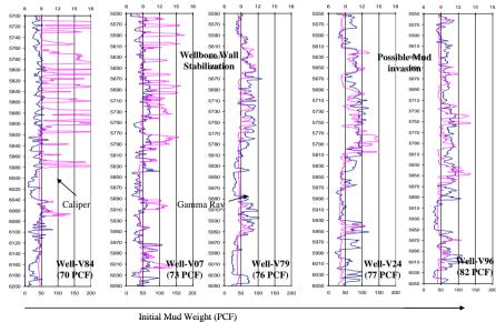
Figure 5. Open hole caliper log of selected vertical wells showing wellbore wall support and possible mud invasion.
