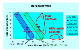
Figure 10. Hole enlargement versus initial mud weight of horizontal wells – identification of mechanisms and design of safe mud weight window.
