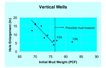
Figure 4. Hole enlargement versus initial mud weight of vertical wells.
