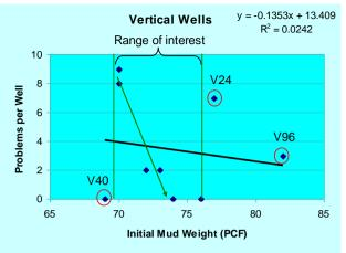
Figure 1. Problems per well versus initial mud weight of vertical wells.
