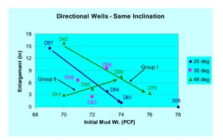
Figure 8. Hole enlargement versus initial mud weight of directional wells studied with respect to inclination angle.
