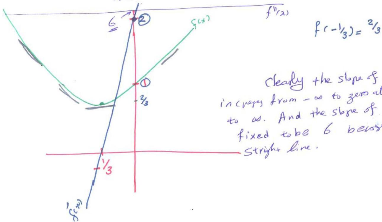
Clearly the slope of  $f(x)$  increases from  $-\infty$  to zero at  $-1/3$  then to  $\infty$ . And the slope of  $f'(x)$  is fixed to be 6 because it is straight line.
