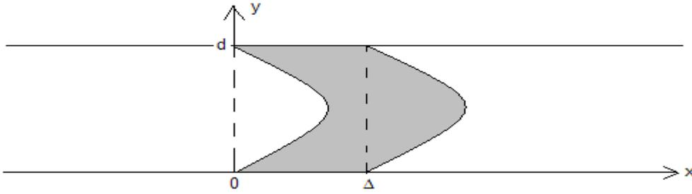
Figure 1(b) - Schematic of a configuration a short time ( $t < \Delta/u_{\max}$ ) after dispersion and advection begins.
