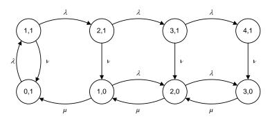
Figure 1. Markov state transition diagram for modeling interrupt disable-enable scheme
