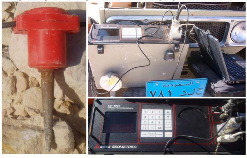
We used the geophone (receiver) and the seismograph (recorder) to conduct our measurements of seismic refraction and refraction micotremor which means recording the noise. Considering the instrument which is old (more than 15 years), it does work.
