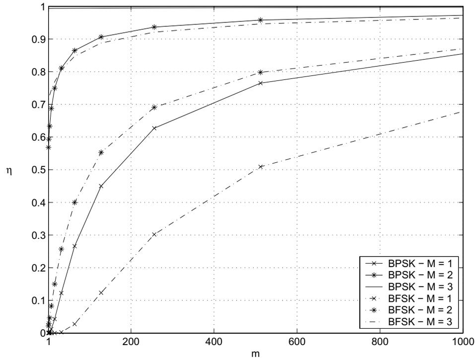
Figure 4. Throughput of SR ARQ systems employing coherent BPSK and noncoherent orthogonal BFSK modulation schemes over Nakagami block fading channels at  $\gamma_s = 15$  dB versus the block length  $m$  for a packet length of  $N = 1024$ .
