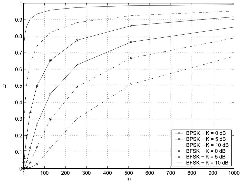
Figure 2. Throughput of SR ARQ systems employing coherent BPSK and noncoherent orthogonal BFSK over Rician block fading channels at  $\gamma_s = 15$  dB versus the block length  $m$  for a packet length of  $N = 1024$ .
