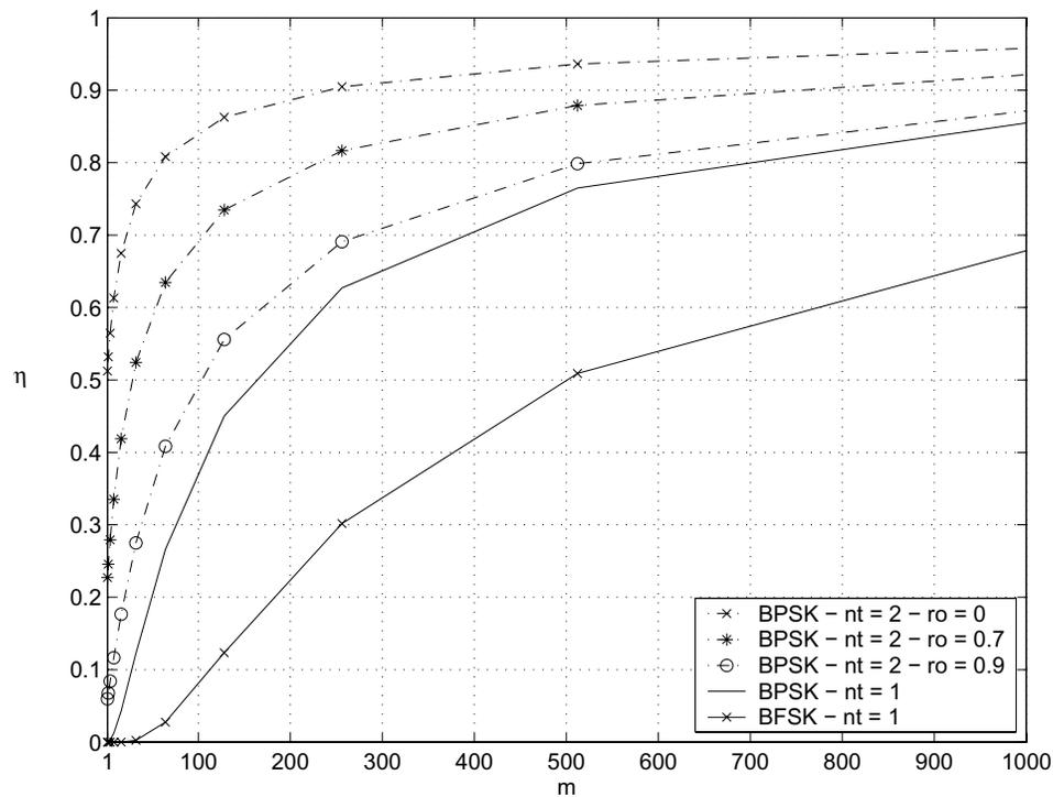
Figure 6. Throughput of SR ARQ systems employing different modulation schemes over Rayleigh block fading channels at  $\gamma_s = 15$  dB versus the block length  $m$  for a packet length of  $N = 1024$ .
