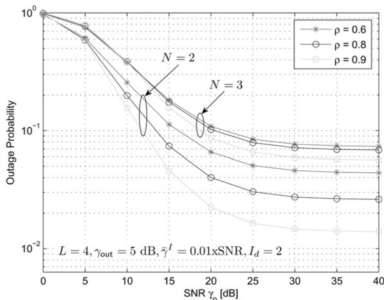
**Fig. 4** Outage probability against SNR for diversity systems with  $N$ th-best antenna selection and CCI for different values of  $N, \rho$
