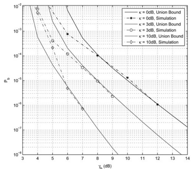
Figure 4 Bit error probability of a convolutionally encoded BI-STCM using  $n_T = 2$  over Rician fading channels with different  $\kappa$  values
