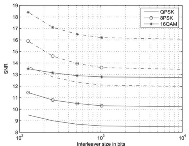
**Figure 8** SNR required to achieve a BER of  $10^{-6}$  against the interleaver size for convolutionally encoded BI-STBC and BI-STCM systems employing  $n_T = 2$  with different modulation schemes under Rayleigh fading (solid: BI-STBC, dashed: BI-STCM)
