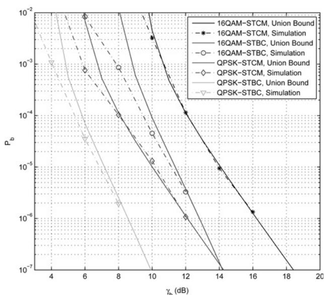
Figure 2 Bit error probability of convolutionally encoded BI-ST systems using  $n_T = 2$  under Rayleigh fading
