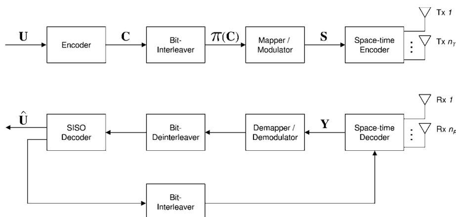
Figure 1 Block diagram of the general BI-ST coded system
