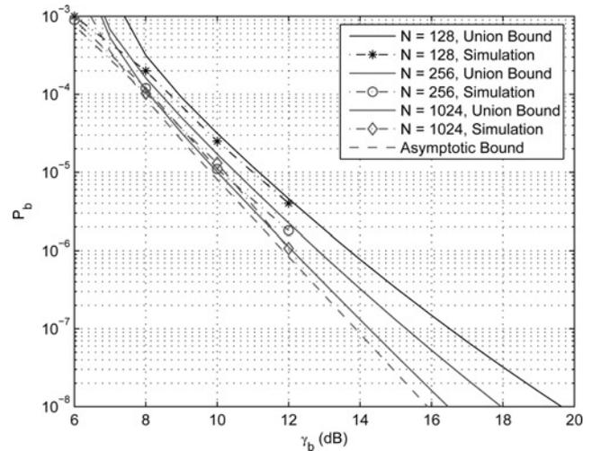
**Figure 7** Bit error probability of a convolutionally encoded BI-STCM using  $n_T = 2$  under Rayleigh fading with different interleaver sizes
