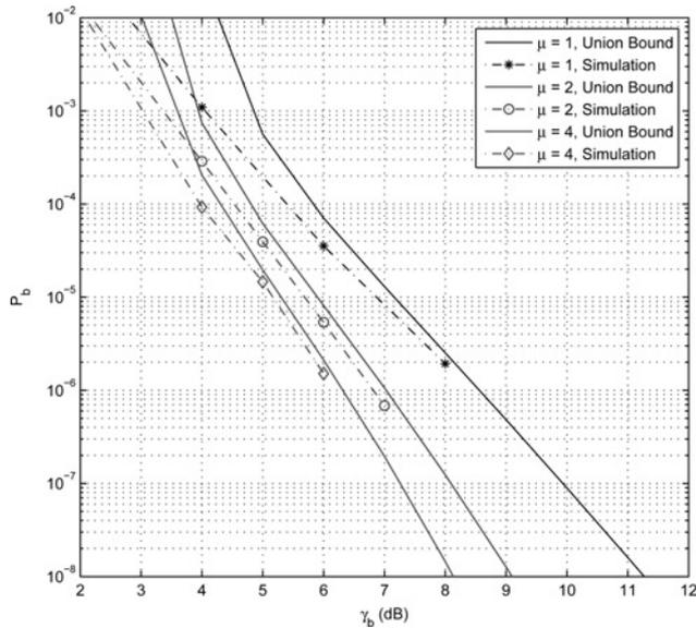
**Figure 5** Bit error probability of a convolutionally encoded BI-STBC using  $n_T = 2$  over Nakagami fading channels with different  $\mu$  values
