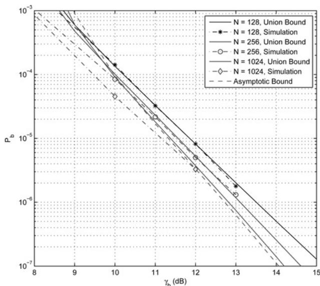
**Figure 6** Bit error probability of a convolutionally encoded BI-STBC using  $n_T = 2$  under Rayleigh fading with different interleaver sizes
