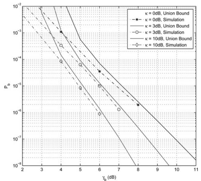
Figure 3 Bit error probability of a convolutionally encoded BI-STBC using  $n_T = 2$  over Rician fading channels with different  $\kappa$  values
