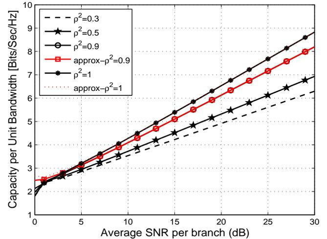
Fig. 2. Capacity per unit bandwidth for a Rayleigh fading with MRC diversity ( $L=3$ ) and various values of different  $\rho^2$  under constant power and rate adaptation
