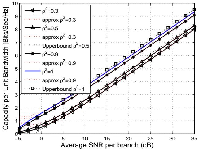
Fig. 1. Capacity per unit bandwidth for a Rayleigh fading with SCD diversity ( $L=3$ ) and various values of different  $\rho^2$  under power and rate adaptation
