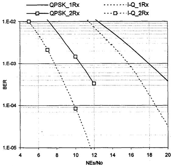
Figure 4: Performance of the 4-state QPSK codes for 1-Rx and 2-Rx antenna over correlated fading channel with  $f_D T=0.01$ .
