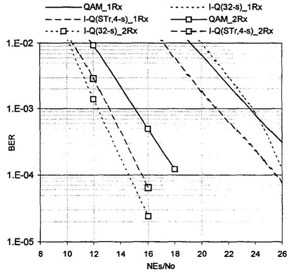
Figure 5: Performance of the 16-QAM codes for 1-Rx and 2-Rx antenna over independent fading channel. STr: Super Trellis.
