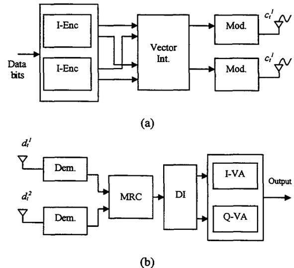
Figure 1: The structure of an I-Q ST system using two transmit antennas.
