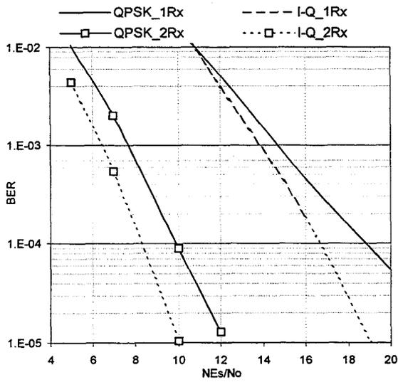
Figure 3: Performance of the 8-state QPSK codes for 1-Rx and 2-Rx antenna over rapid fading channel.
