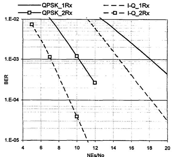
Figure 2: Performance of the 4-state QPSK codes for 1 and 2 Rx antennas over independent fading channels.
