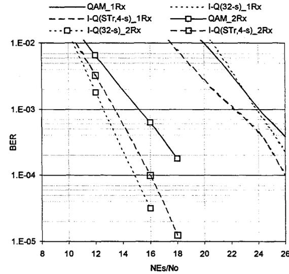
Figure 6: Performance of the 16-QAM codes for 1-Rx and 2-Rx antenna over correlated fading channel with  $f_D T=0.01$ .
