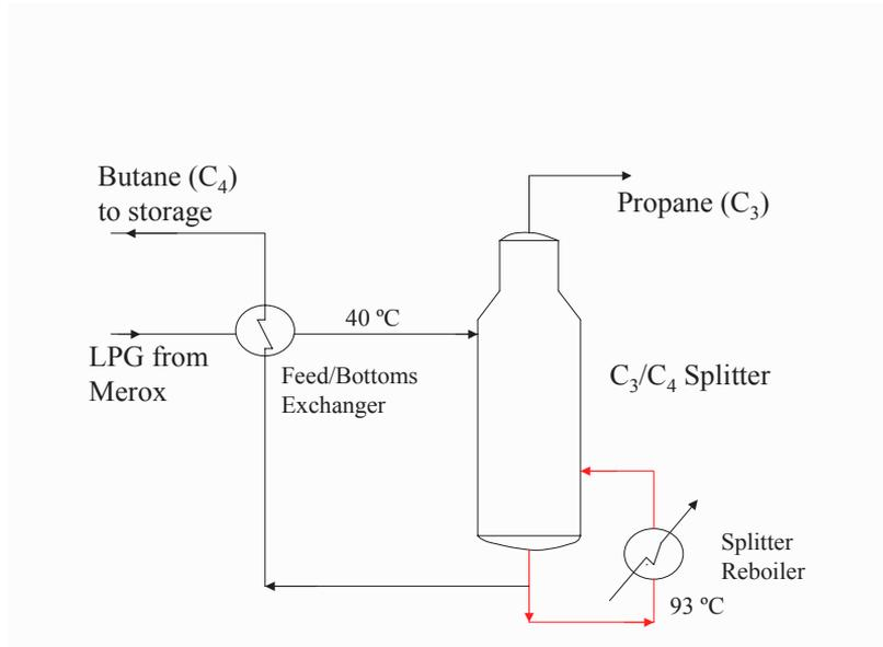
Fig. 5: simplified flow diagram of LPG Splitter
