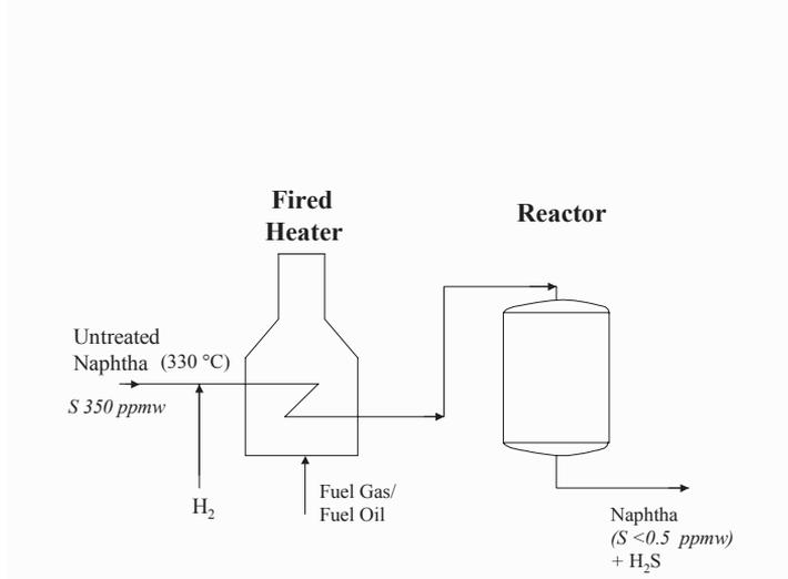
Fig. 1: simplified flow diagram of Naphtha Hydrotreater unit
