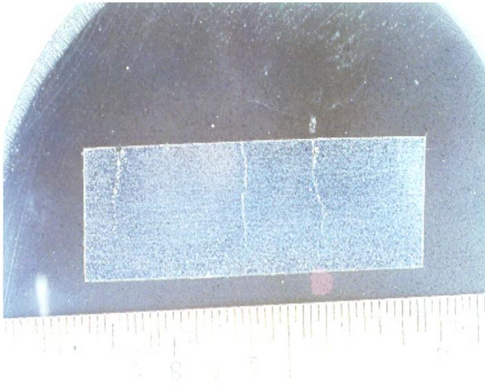
Fig. 3: cracking from ID surface (top)
