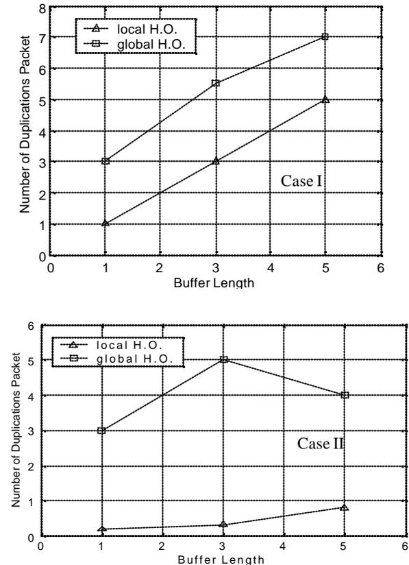
Fig.7: Duplicated packets versus buffer length (a) Case I (b) case II
