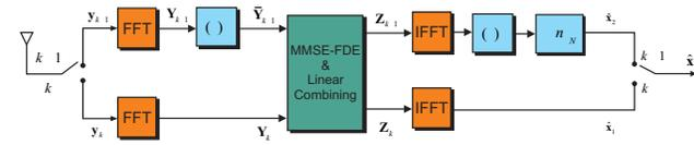
Figure 4: Block Space-Time Coding for frequency selective Channels: Receiver
