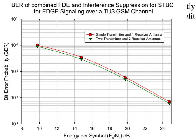
Figure 7: BER of combined FDE and Interference Suppression for STBC for EDGE Signaling over a TU3 GSM Channel
