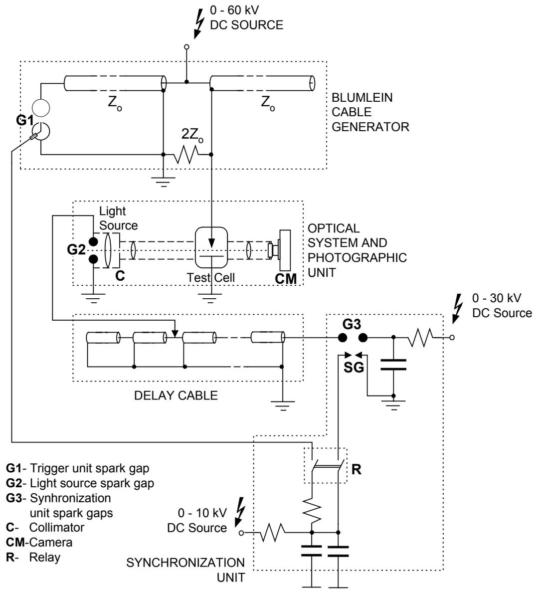
Figure 1. The experimental set-up.
