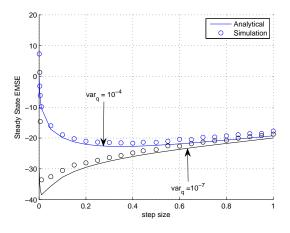
Fig. 2. Analytical and experimental steady state EMSE vs step sizes with  $\text{Tr}(\mathbf{Q}) = 10^{-4}, 10^{-7}$  with  $\alpha_c = 0.7$  and  $\epsilon = 0.05$ .
