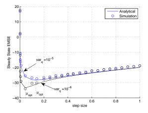
Fig. 4. Analytical and experimental steady state EMSE vs step sizes indicating  $\mu_{\rm opt}$  for  $\text{Tr}(\mathbf{Q}) = 10^{-5}, 10^{-6}$  with  $\alpha_c = 0.2$  and  $\epsilon = 0.001$ .
