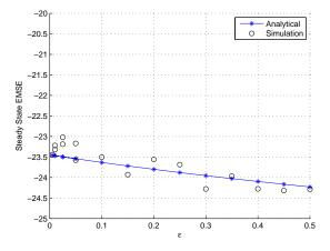
Fig. 3. Analytical and experimental steady state EMSE vs epsilon  $Tr(\mathbf{Q}) = 10^{-5}$ ,  $\alpha_c = 0.2$  and  $\mu = 0.6$ .
