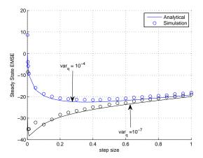
Fig. 1. Analytical and experimental steady state EMSE vs step sizes with  $\text{Tr}(\mathbf{Q}) = 10^{-4}, 10^{-7}$  with  $\alpha_c = 0.2$  and  $\epsilon = 0.05$ .
