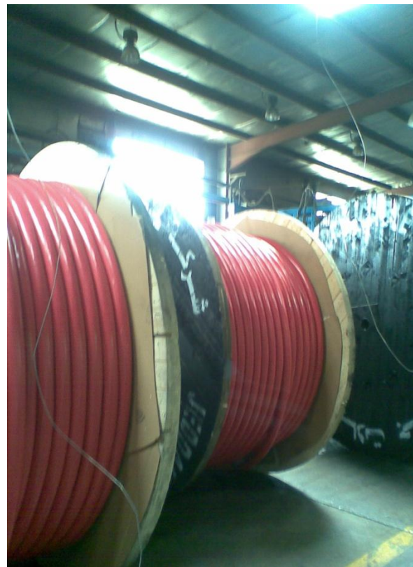
Figure 12: Final Cable Products after Sheathing
