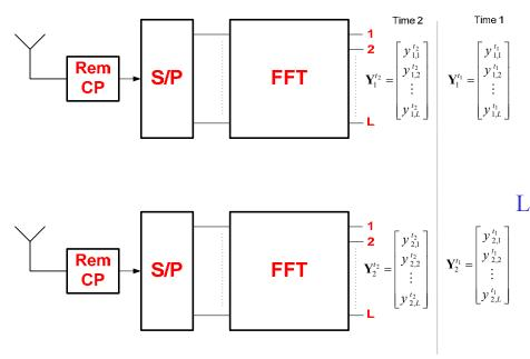
The received vectors over two time periods at the output of the FFT is
