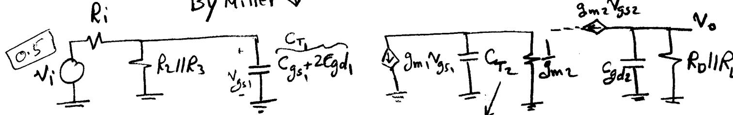
$$\omega_{H1} = \frac{1}{R_{C_T1} C_{T1}} = \frac{1}{(R_i || R_2 || R_3)(C_{gs1} + 2C_{gd1})} = 73.226 \text{ rad/s} \Rightarrow f_{H1} = 11.65 \text{ MHz}$$
