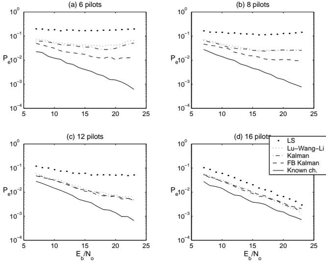
Fig. 3. Comparing the BER curves for various receivers.
