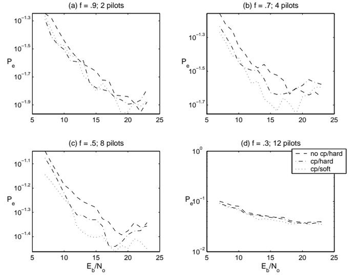
Fig. 2. The FB-Kalman based receiver demonstrates improved BER with increasing levels of signal processing
