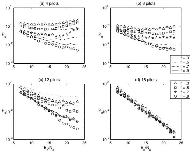
Fig. 1. Comparing the Kalman and FB-Kalman for various levels of time-variation (Solid and dotted lines are for the Kalman receiver).
