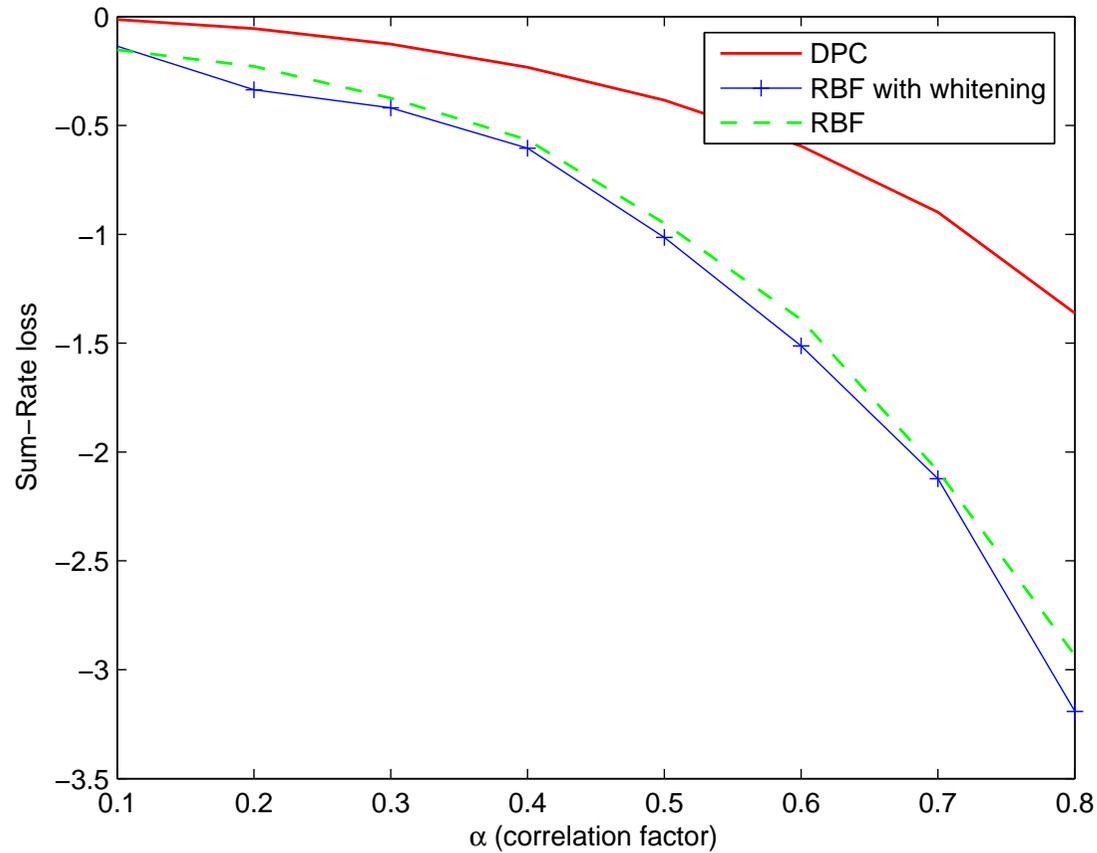
Figure 2: Sum-rate loss versus the correlation factor  $\alpha$  for a system with  $M = 3$  and  $n = 100$ .
