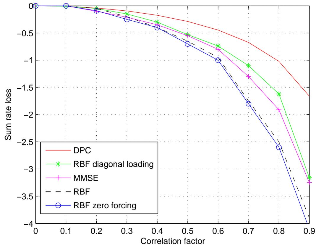
Figure 5: Sum-rate loss versus correlation factor  $\alpha$  for a system with  $M = 3$ ,  $P=10$  and  $n = 200$ .
